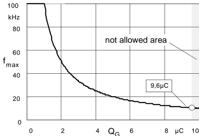
Fig.14 Maximum operating frequency x gate charge
