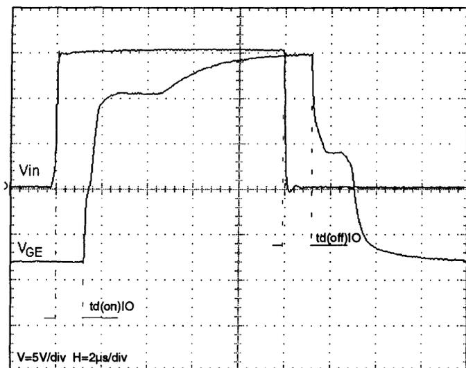
Fig. 10 Input and output voltage propagation time
