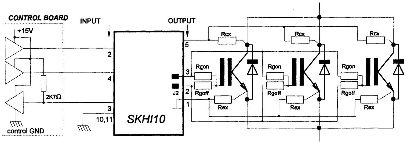
Fig. 9 Preferred circuit for paralleled IGBT's
