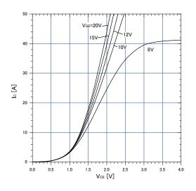
Graph.5 Typical Transfer Characteristics  $V_{\text{GE}}$ =+15V
